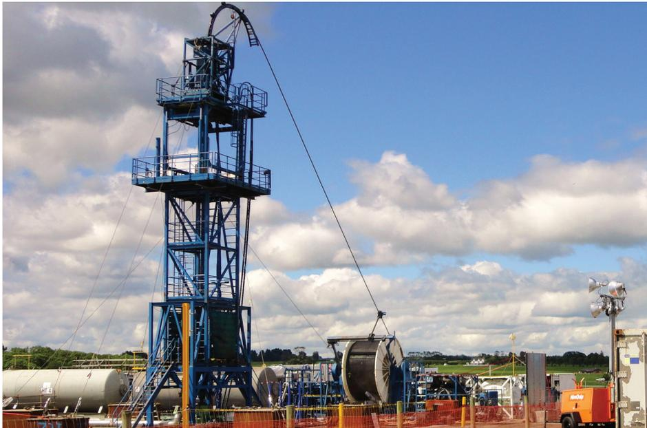
An onshore Pohokura field well located in Taranaki, New Zealand, exhibited reduced production rates due to scale deposition across the perforated zones. An acid wash delivered via coiled tubing (CT) was planned to remove the scale and any other wellbore debris. The operator wanted the ability to run real-time production logging tools (PLT) following the treatment to confirm the effectiveness of the acid wash.
